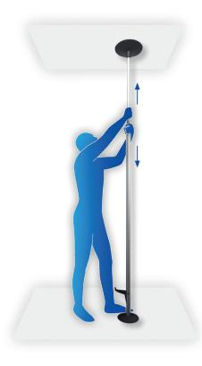
Set the bar on the base plate and put the top plate in place.
