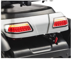
LED lighting system
