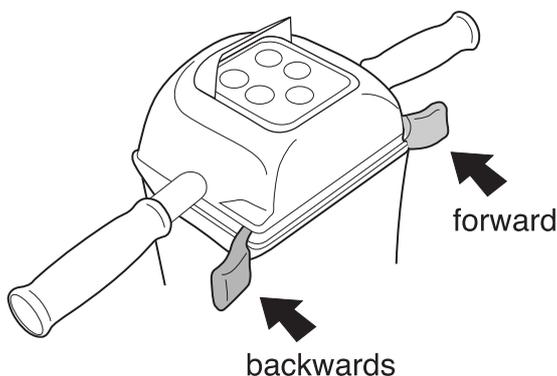
**Forward/Reverse:** Push the right lever to move forward, push the left lever to move backwards.
