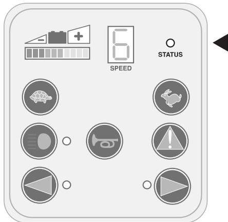
**Status Indicator:** When the scooter is on, and all conditions are normal, the Status Indicator will be on. When there is some special condition that needs attention, the light will flash. See the reference chart below for the meanings of the different flashing patterns.
